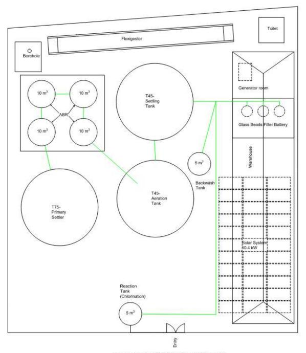
Figure: Layout of FSM Plant at Camp 19
