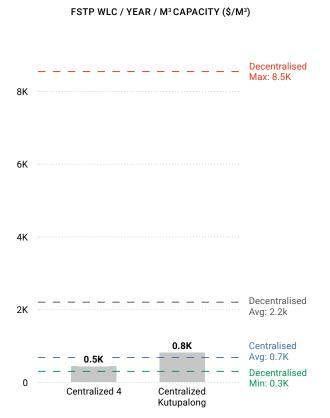
Figure 24: Relative performance of Centralised plants in regard to WLC per volume treated
