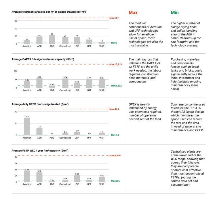
The centralised plants proved to be performing above average while treating to a relatively good standard. This treatment technology can also cope with a wider range of variation of incoming sludge, which caters for the diverse transportation modes currently used in CxB.
