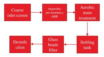
Similar process. Only difference is in the sludge from the settling tank that will goes to drying beds and get incinerate/ flexigester
