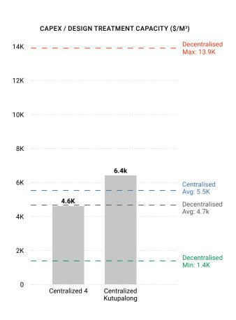
Figure 22: Relative performance of Centralised plants for Capex (per m<sup>3</sup> design treatment capacity)
