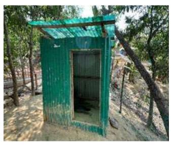
Figure 3: Direct pit single cubicle latrine example
