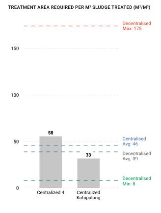
Figure 21: Relative performance of Centralised plants for treatment area required (per m³ of sludge treated)
