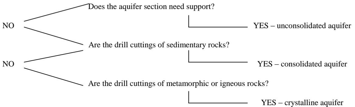
Finally: geophysically log the borehole to confirm the aquifer classification
