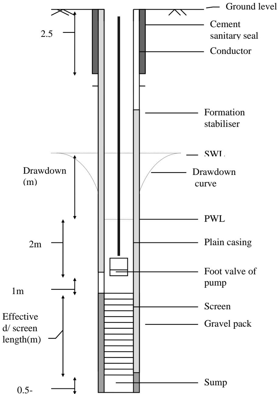
**Sanitary seal** <sup>(12)</sup> very important to avoid contamination of the well from the surface and <sup>(7)</sup> to be 2.5m deep (in the least impermeable layer) with cement plug and **conductor casing**.
