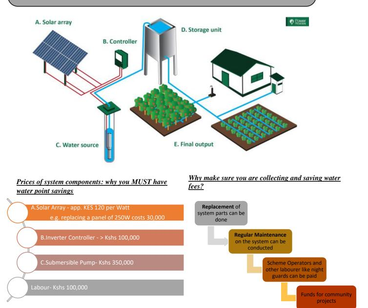
\*\* These are estimated values for a system with 130m total dynamic head and a yield of 8m<sup>3/</sup>hr. System Component costs normally depend on the size of the array as well as the type of pump used.
