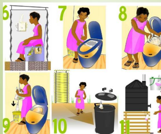
Figure 16: IEC used to explain proper removal of bag from UD toilet and deposit for collection and disposal
