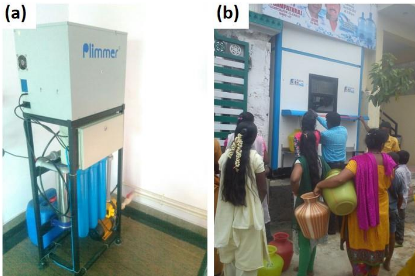
Figure 16: Idropan's mCDI technology: a) Idropan/AquaSphere Plimmer mCDI unit in an Indian hostel; b) community members collecting water from a Plimmer kiosk outside a mosque.
