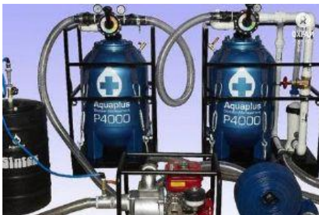
Figure 10- Aquaplus water treatment unit
