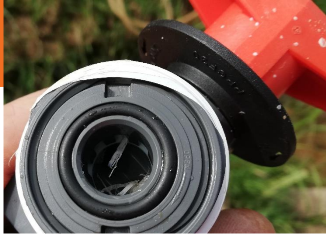
Blockage in dosing flow regulator
