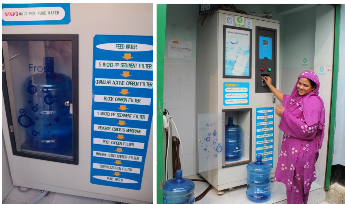
Figure 8 – A coin operated water ATM with integrated treatment, Dhaka
